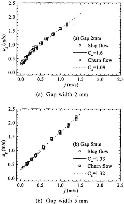
Fig. 5 Drift-flux correlation of the void fraction.
